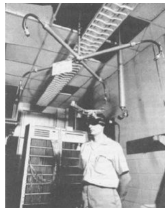
Fig. 2.1 Sutherland, I.E. (1968): A Head -Mounted Three-Dimensional Display
