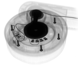
Fig. 2.18 Suovanen, J. (Creative Electron, 2018): Radiography of the HTC Vive Pro headphone
