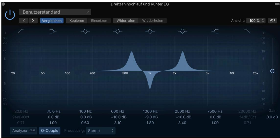
Abb. 4.5 Equalizer Motorensamples<sup>105</sup>
